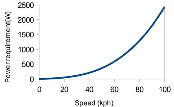
Figure 1. Power dependency on speed.
